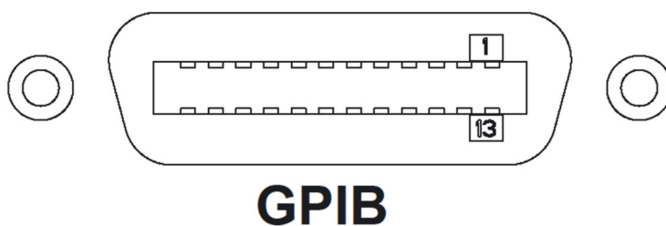
Figure 3-23: GPIB interface Connector
