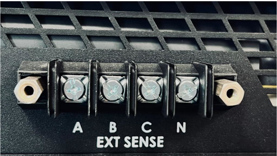
Figure 3-8: External sense Connector
