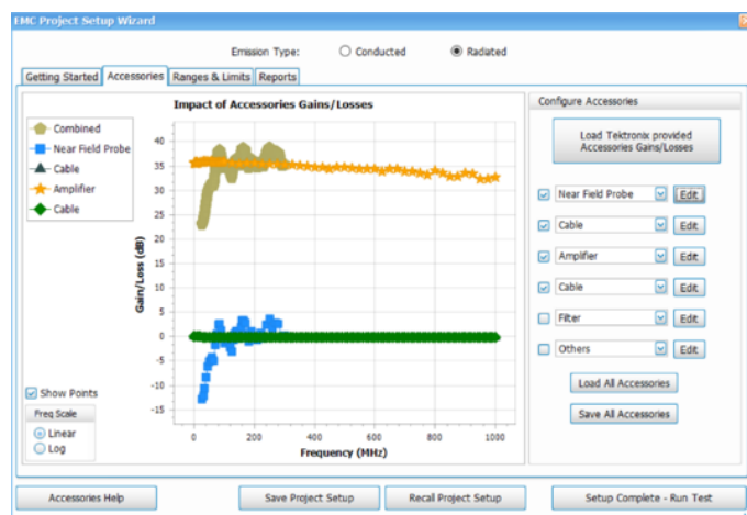
FIGURE 11. For antennas enter either the isotropic gain or Antenna factor.
