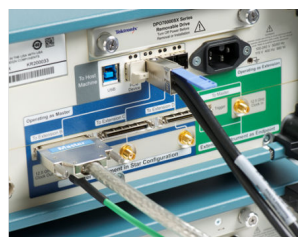
UltraSync connection on instrument with Master role
