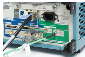
UltraSync connection on instrument with Extension role
