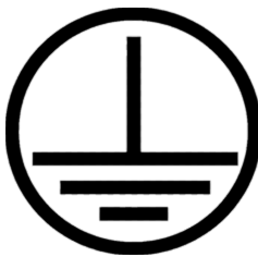
Figure 1.5: Protective Earth (PE) Ground. Indicates the wiring terminal must be connected to 'earth ground' before operating the equipment – for protection against electrical shock in case of a fault
