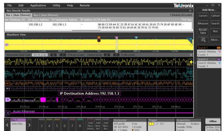
Figure 21: 100BASE-T1 Protocol decode on PC based TekScope Application
