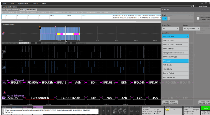
Figure 19: Automotive Ethernet Protocol Decode for full-duplex ECU
