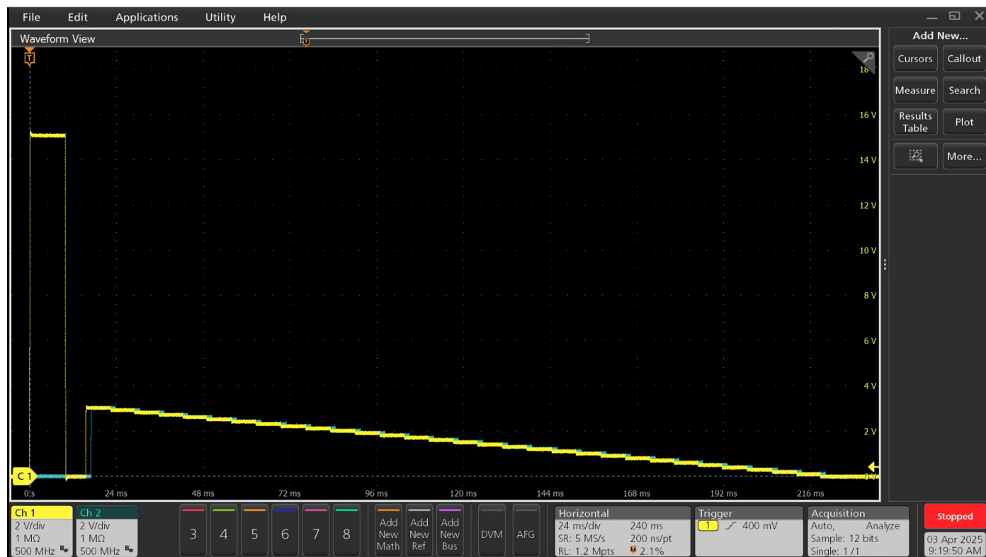
Figure 11. Oscilloscope capture of sic-mosfet-vth-vgvdswEEP-smu test.
