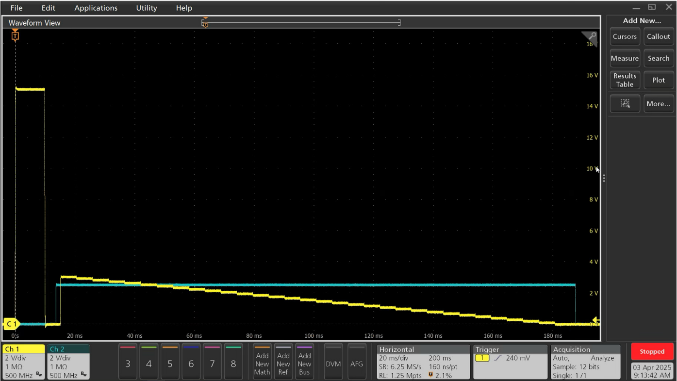
Figure 7. Oscilloscope Capture of sic-mosfet-vth-vgsweep-vdfixed-smu test.
