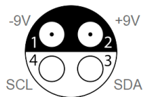
Probe's power supply pin assignment "cable view"
