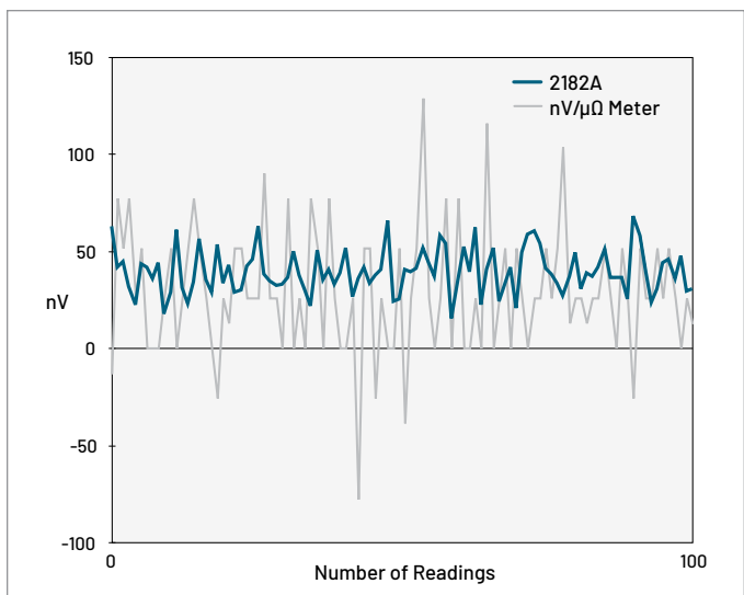
Figure 1. Compare the 2182A's DC noise performance with a nanovolt/micro-ohmmeter's. All the data shown was taken at 10 readings per second with a low thermal short applied to the input.
