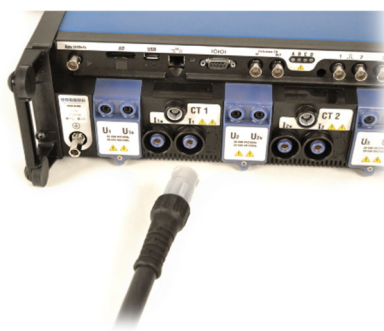
Figure 5.1 Installing locking style connectors.
