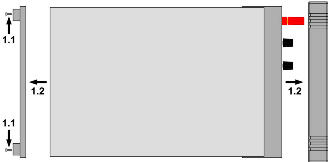
Figure 7 - Removal of the front and rear frame
