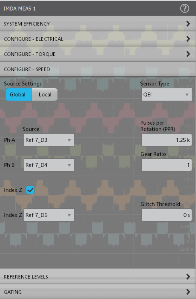
Configuration options for computing System Efficiency using QEI method.
