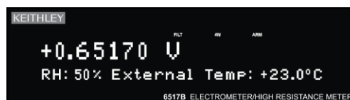
Figure 7: Relative humidity and external temperature display
