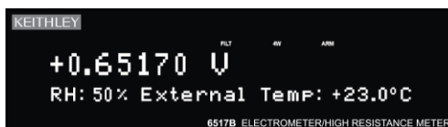
Figure 43: Relative humidity and external temperature display
