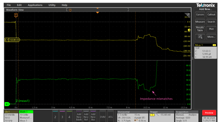
The TDR analysis provides an impedance waveform for the trace in the above figure. The impedance, capacitance and inductance of the waveform across marked regions are displayed in a measurement badge. The lower impedance in the center of the screen corresponds to the wider section of the PCB trace.
