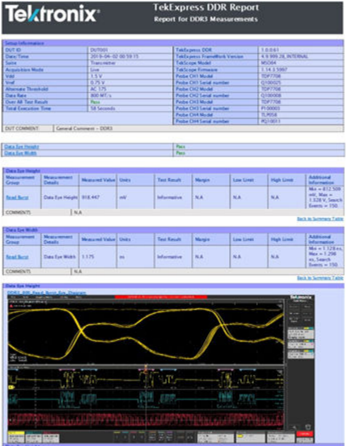
6-CMDDR3 Report file with DDR3 Eye diagram test result.
