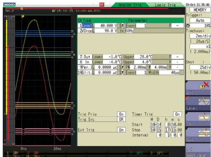
Adjust levels while displaying waveforms
