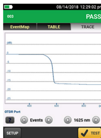
Splitter as seen on an OTDR trace
