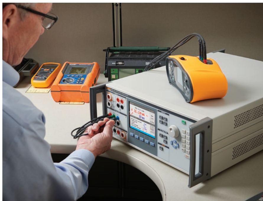
Each 5322A comes with an external R-Multiplier to source resistances of 10 TOhm for testing insulation testers.
