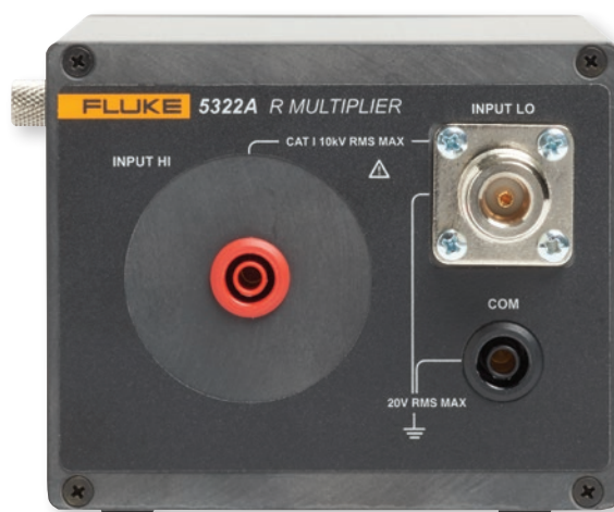
Each 5322A comes with an external R-Multiplier to source resistances of 10 TOhm for testing insulation testers.
