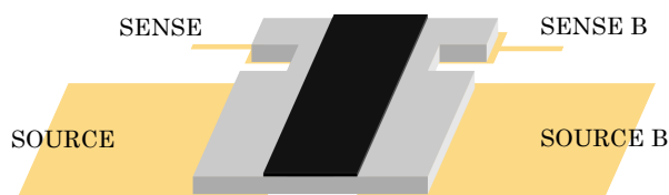
Figure 2. Connections Using Mounted Patterns
