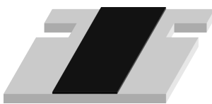
Figure 1. Shunt Resistor Shape
