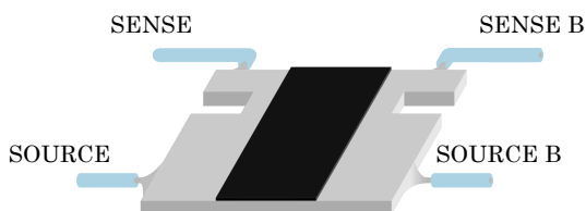
Figure 3. Connections Using Lead Wires
