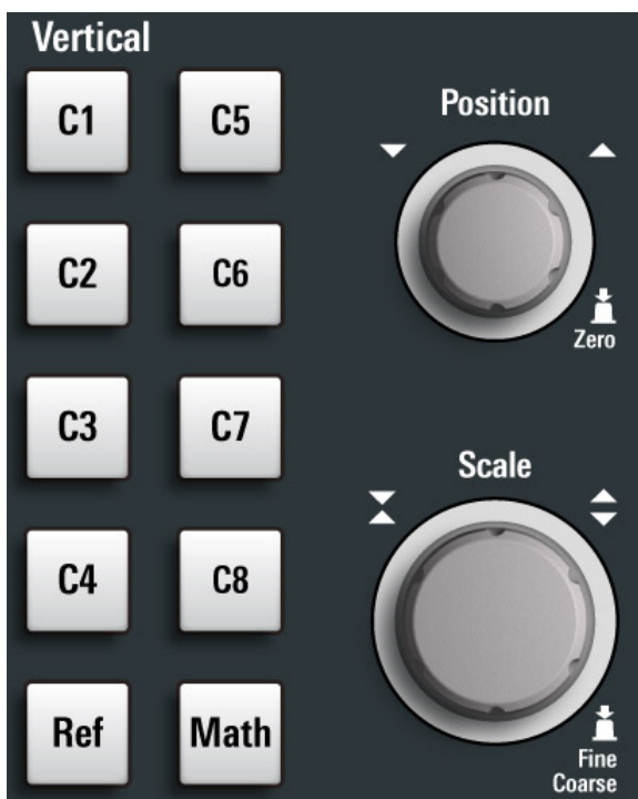
Figure 5-5: Vertical controls of MXO 5 with 8 input channels
