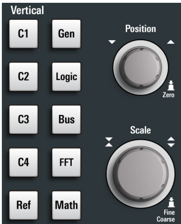
Figure 5-4: Vertical controls of MXO 5 with 4 input channels
