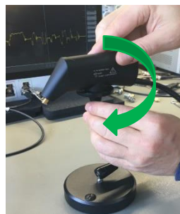
Twist by 90° to mount or unmount
