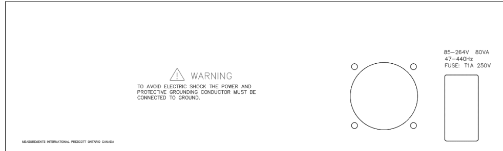
Figure 7-2. 1340A Rear Panel Connection Terminals.
