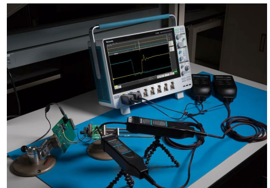
FIGURE 4. Many power supply topologies require measurements of small differential voltages in the presence of high common mode signals. For example, V_{GS} and V_{DS} on the high side of a half-bridge switching stage often move up and down 100s or 1000s of volts relative to ground. IsoVu™ Isolated Measurement Systems offer extremely high common mode rejection.
