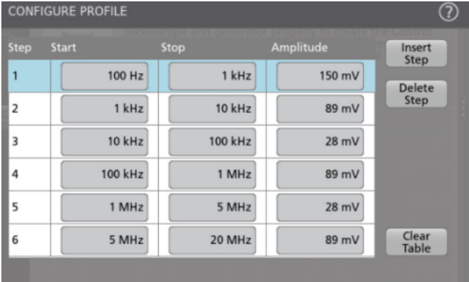
FIGURE 19. An amplitude profile may be used to improve signal-to-noise ratio (SNR) of measurements. It enables application of lower amplitudes at frequencies where the DUT is sensitive to disturbances and higher amplitudes at frequencies where it is less sensitive.
