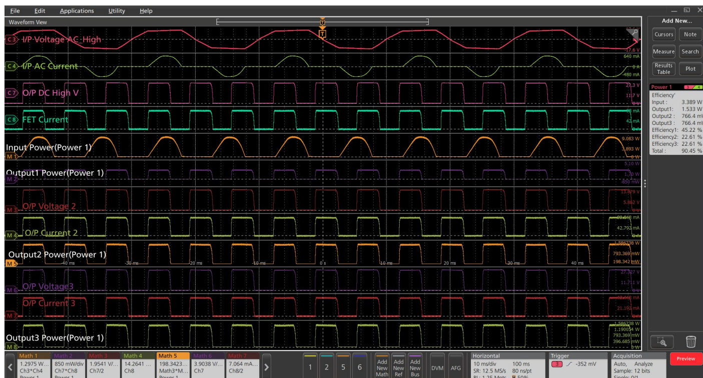
FIGURE 27. Efficiency measurement in which a single AC voltage and current are used to determine input power, and power is measured on three outputs simultaneously to find total efficiency.
