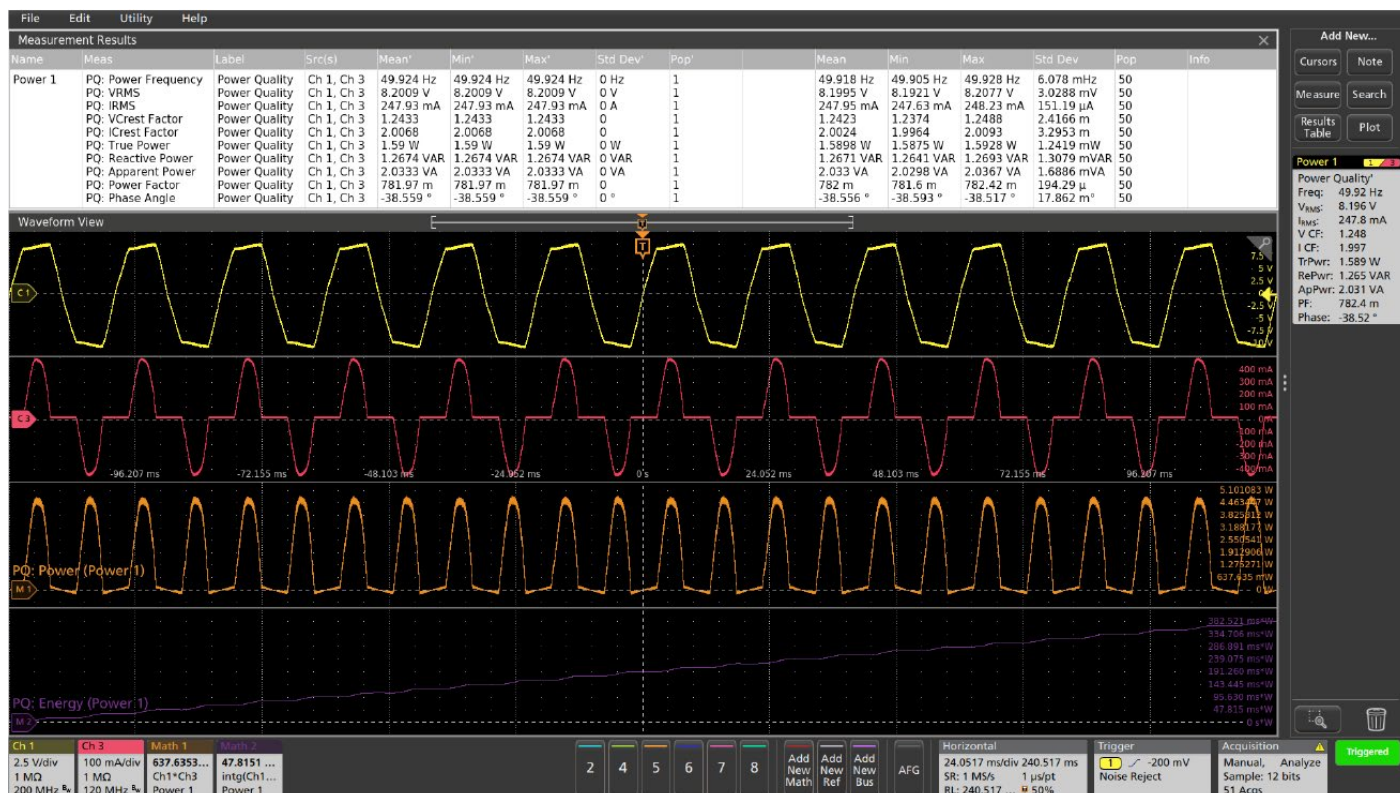
FIGURE 5. Power quality measurements paint a rich picture of the AC line. Line voltage is the upper waveform. Current is the red waveform. Instantaneous power is the orange waveform. The results badge (upper right) shows a summary of the line characteristics, and the results table in the upper section can be activated for more detailed data and statistics.
