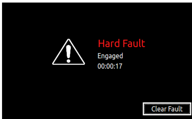
Figure 3-103. Hard Fault Screen
