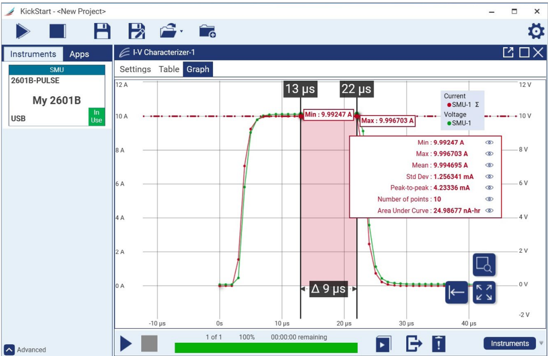
Figure 14: Analysis example of a pulse within KickStart.
