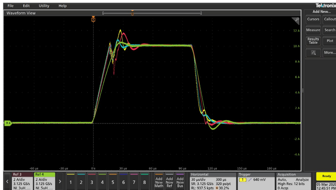
Figure 15: Pulse outputs that have overshoots and undershoots due to cable inductances.
