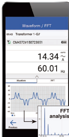
Waveform observation, FFT analysis
