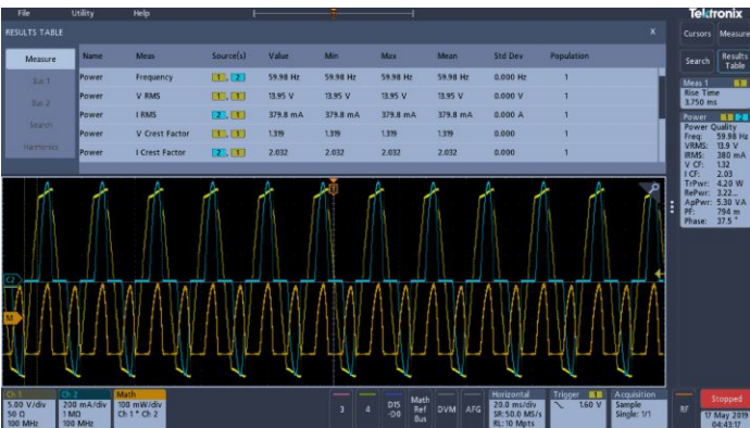
Power quality measurements
