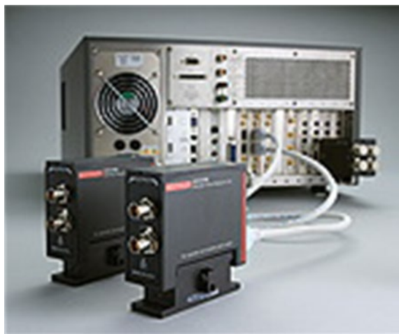
Figure 1: Model 4225-RPM and Model 4200-SCS backplane
