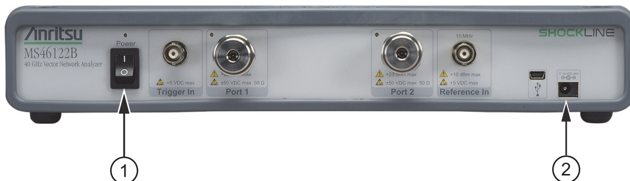
Figure 3-1. Front Panel Power Connection to AC Mains Power
