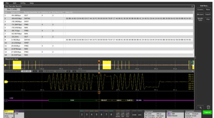
Results table showing all USB HS packet information with time-stamp information
