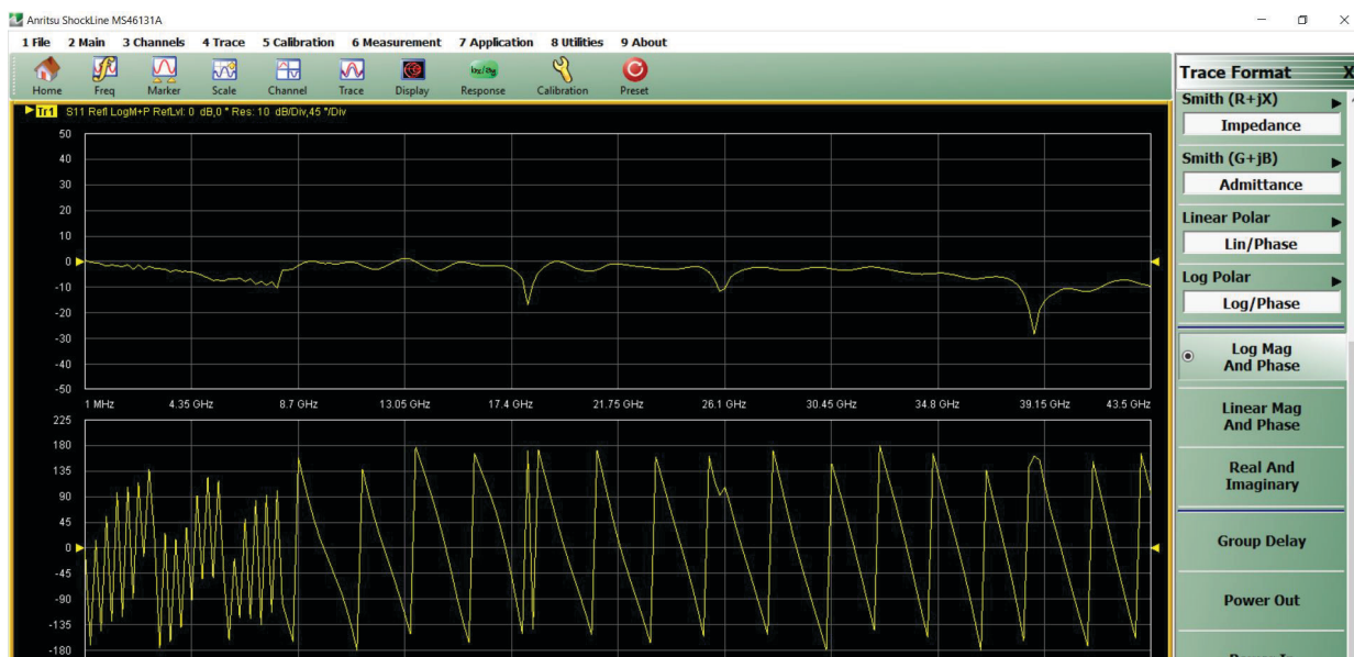
Figure 4-19. Trace Graph - Rectilinear Paired - Trace Log Magnitude and Phase Trace Display
