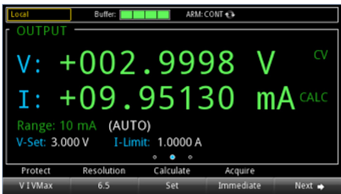
Figure 3. Current readout when the multimeter is not connected
