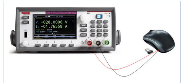
Figure 8. 2280S is connected to the DUT
