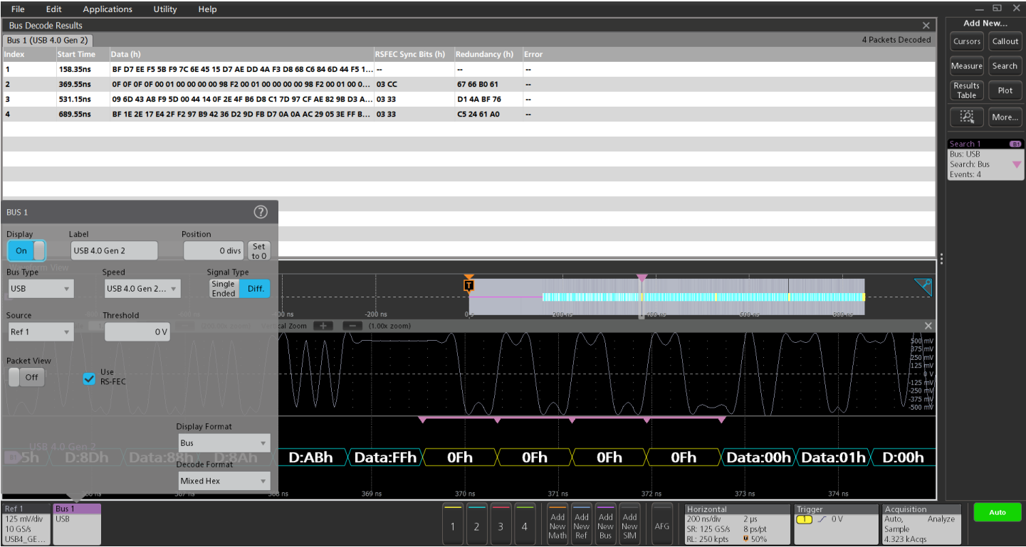
USB4 Gen2 bus setup showing decode with packet view Off with RSFEC. START_RSFEC searched with 4 occurrences.
