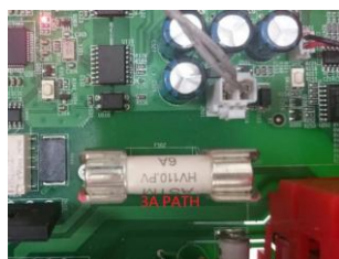
Internal 3A input current fuse
