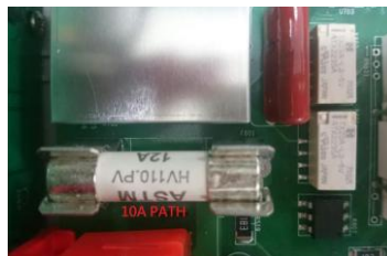
Internal 10A input current fuse
