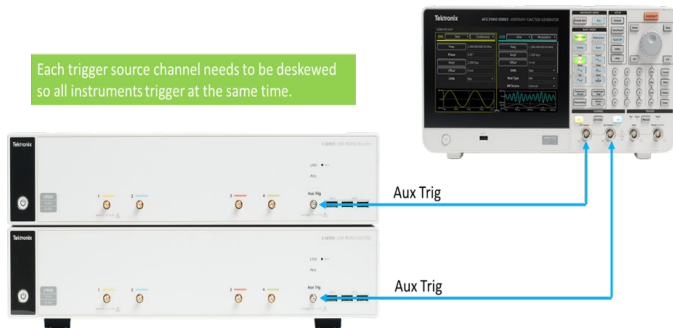
Setup diagram to quickly achieve moderate skew among channels
