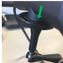
Make sure probe head is fully inserted and seated into holder
