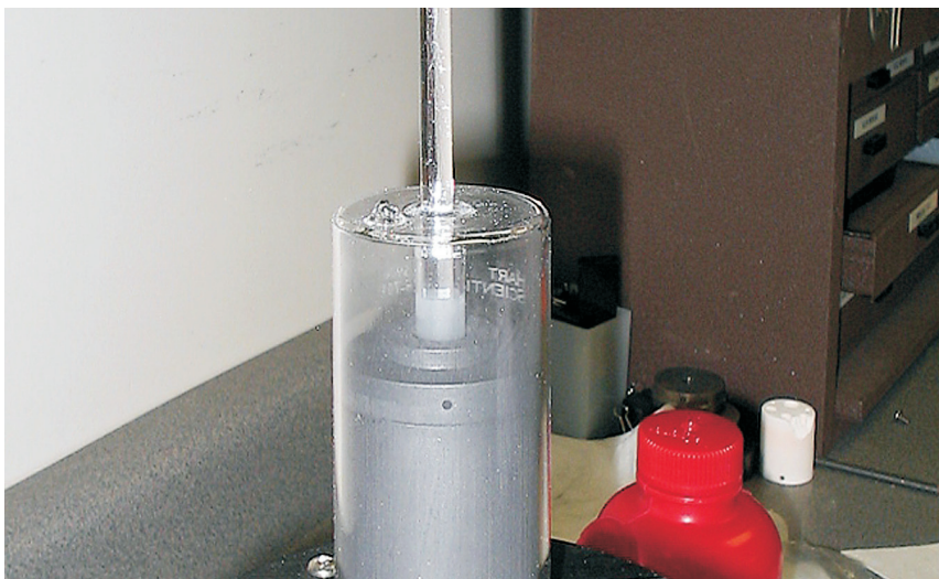
Figure 15 Push insulation to bottom of re-entrant well.
