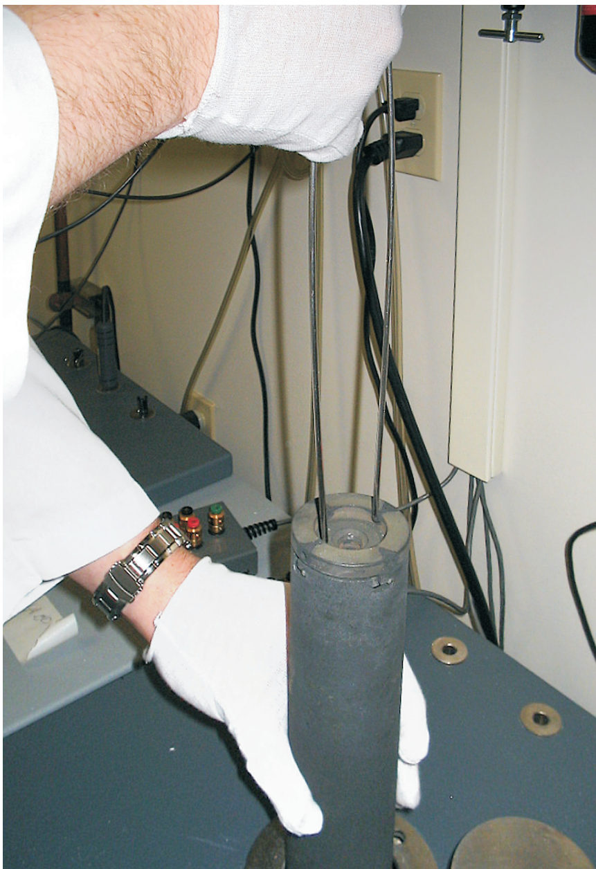
Figure 26 Installing basket assembly in furnace.
