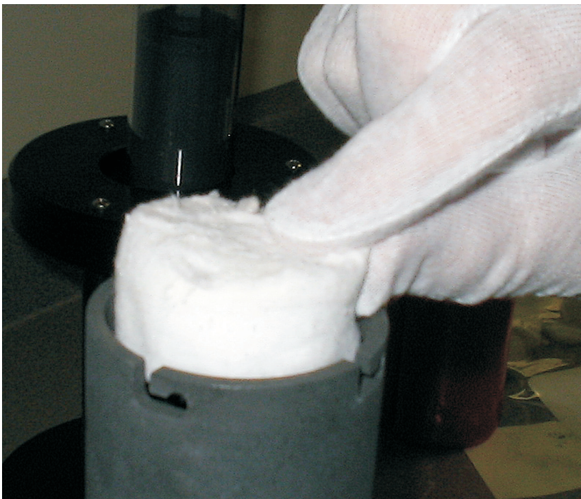
Figure 17 Place insulation in cell basket
