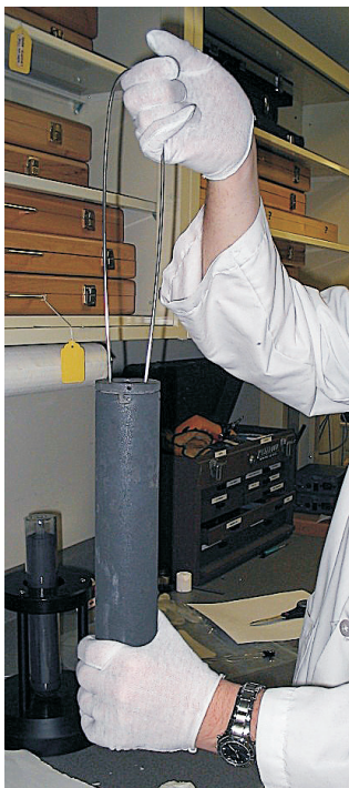
Figure 25 Preparing basket assembly for installation in furnace.
