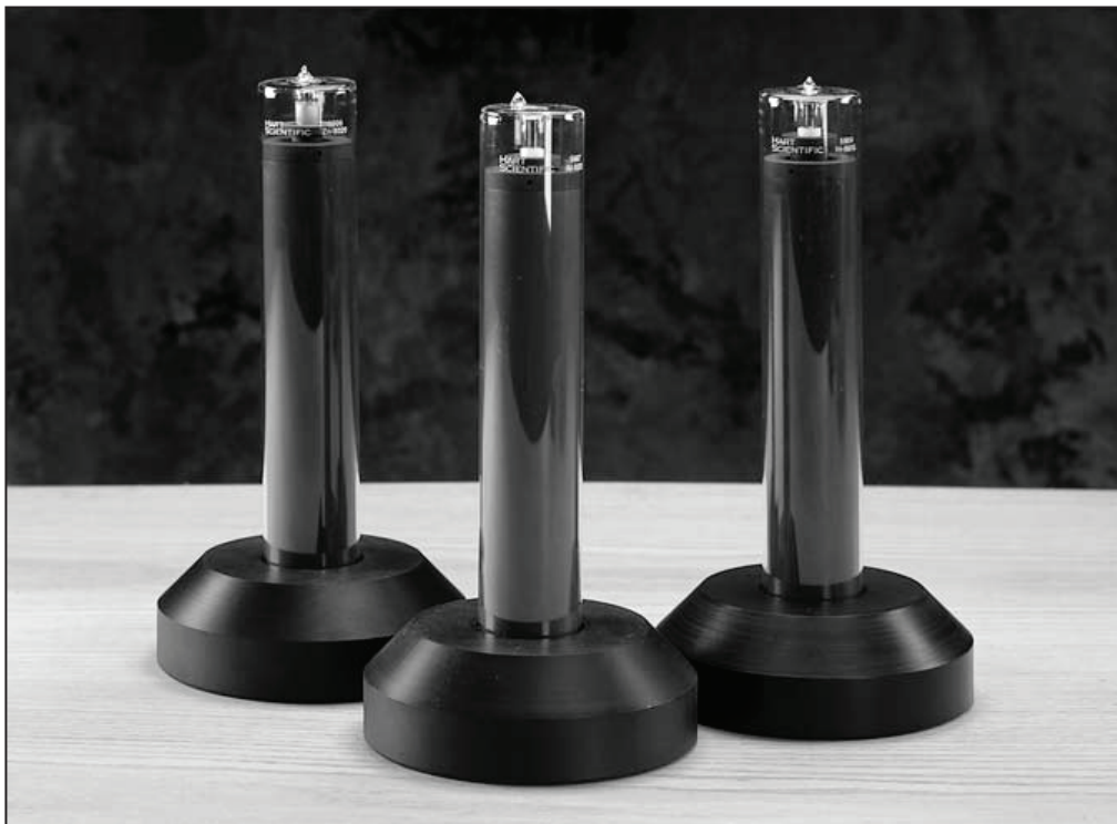
Figure 1. The Metal Freezing Point Cell
