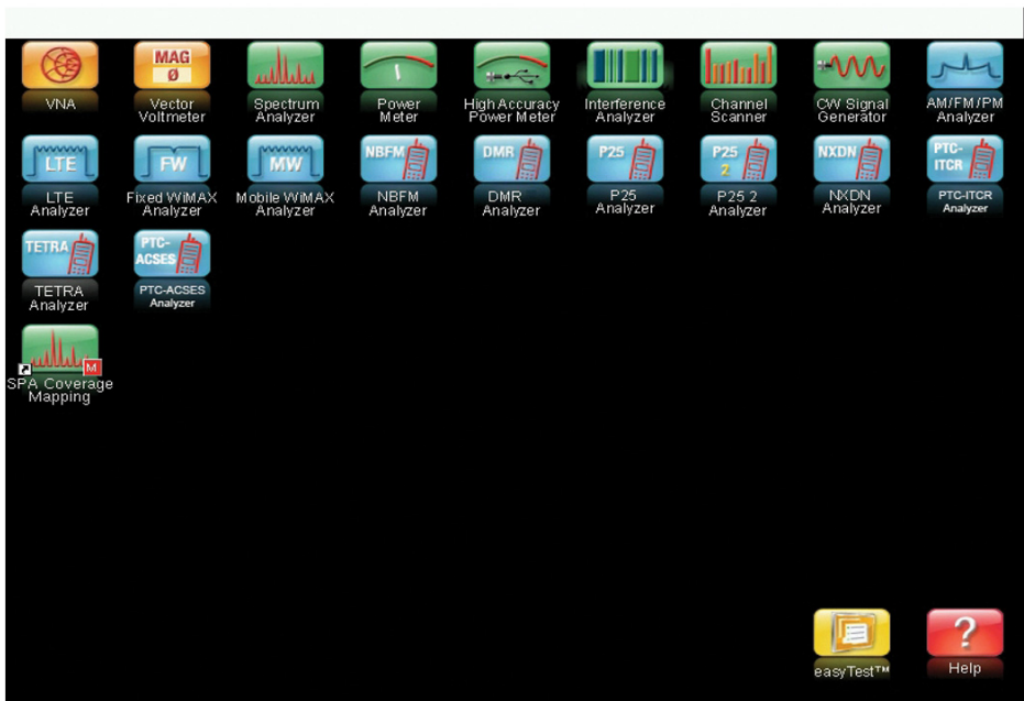
Figure 2-2. Menu Key Screen, Icons for Installed Measurements
