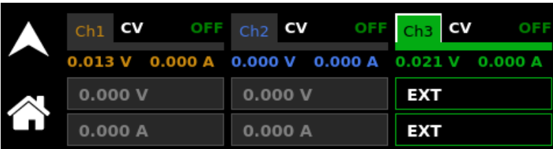
Figure 3-21: Output Voltage and current as EXT Reference Mode for Channel 3
