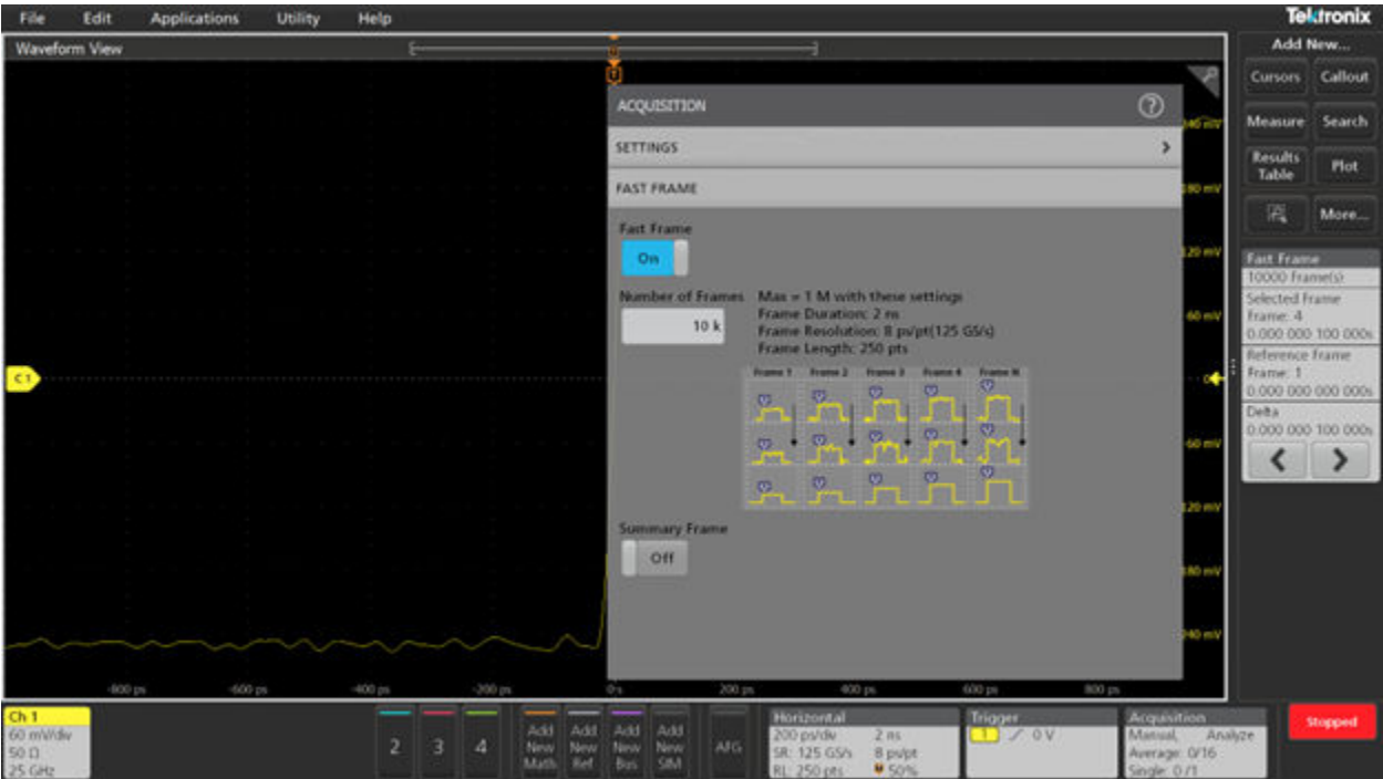
FastFrame™ with Orthogonal Frame Averaging
