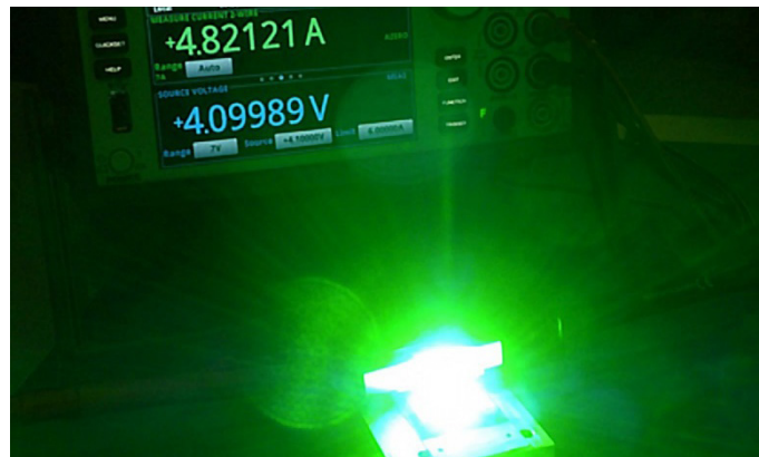
FIGURE 13: HBLED illuminated at 4.1 volts and 4.8 amps.
