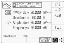
Note that the upper sinewave amplitude range limits are halved by invoking Dual Channel Sine function.
