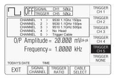
Note that the expected load key in the bottom right corner is now de-activated, and the trigger state legend in the top central box is fixed on  $50\Omega$ . A further selection is available, to choose the trigger ratio.
