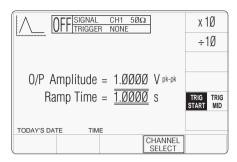
The 9500B has auto-selected a Ramp Time of 1.0000s. Trigger is auto-selected: 'TRIG START', not 'TRIG MID'. O/P Amplitude is fixed at 1.0000V.
