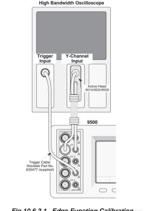
Fig 10.6.3.1 Edge Function Calibration — Interconnections
