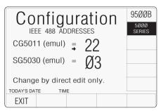
Note that the 9500B contains two IEEE-488 interfaces, each of which will respond to a separate address. 9500B and CG5011 occupy one IEEE bus address and can be modified either on the 9500B screen or the 5000 series screen. SG5030 occupies the other bus address, which can be modified only on the 5000 series screen. The 5ØØØ SERIES selection also switches the interface to accept the emulation commands only.
