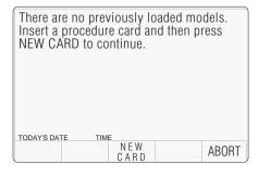
In this case, insert the card required for the UUT into PCMCIA SLOT 1, push gently home, and press the 'NEW CARD' screen key for the sequence to continue.
