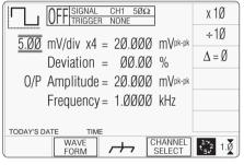
The above default screen has auto-selected the positive square waveform, as indicated by the icon in the top left corner. Frequency is variable between 10.000 Hz and 100.00 kHz. Frequency has defaulted to 1 kHz, deviation ' $\Delta$ ' to zero, and output voltage to 20.000 mVp-p. The Duty Cycle is fixed at a nominal 50%.
