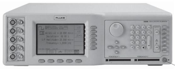
Center: A 'Menu' and 'Output Display' LCD screen, with grouped soft keys.
