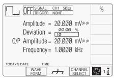
Fig. 4.4.6 Numeric Entry — Effect on Deviation Value and Screen Key Labels
