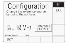
When switched to 'EXT.', use the up/down cursor control or spinwheel to inform the 9500B of the source frequency. Ensure that the required source is connected and operating.
