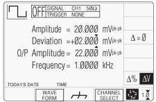
Fig. 4.4.10 Voltage Deviation Applied
