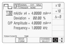
The above default screen has auto-selected the symmetrical square waveform, as indicated by the icon in the top left corner. Frequency is variable between 10.000Hz and 100.00kHz. Frequency has defaulted to 1kHz, deviation  $^{\rm L}\Delta$  to zero, and output current to 4.0000mAp-p. The Duty Cycle is fixed at a nominal 50% .
