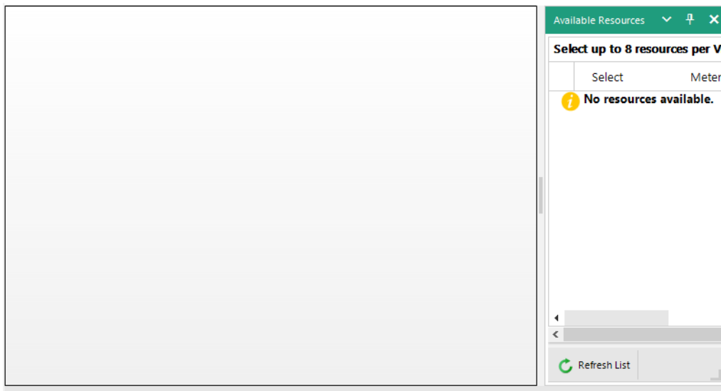
Figure 3-12. Docking a Window to the Right-side of the Main Window
