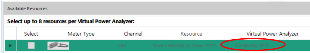
Figure 3-9. The Available Resources Box Shows Assigned Devices
