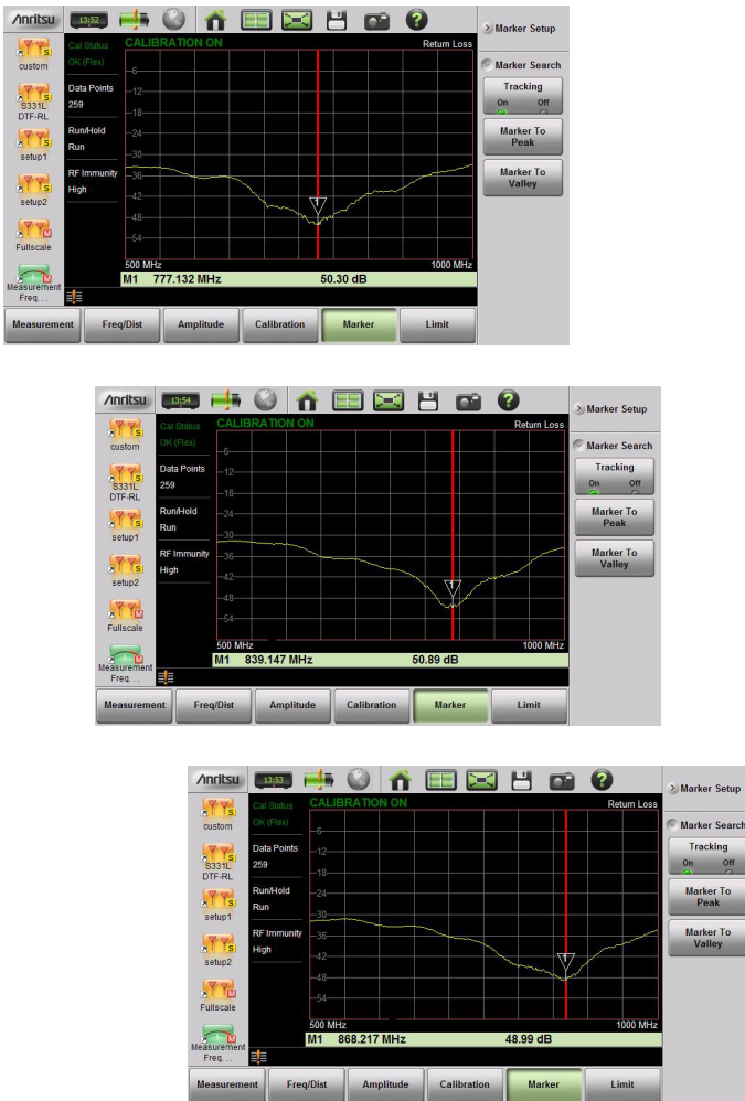
Figure 3-27. Tracking Marker Set to Valley
