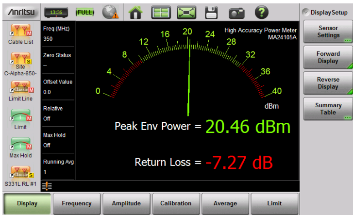
Figure 9-6. Power Meter View
