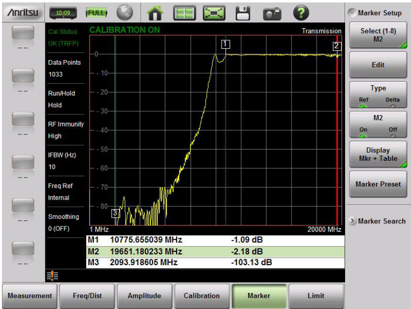
Figure 3-13. 2-Port Transmission Measurement Example, Waveguide
