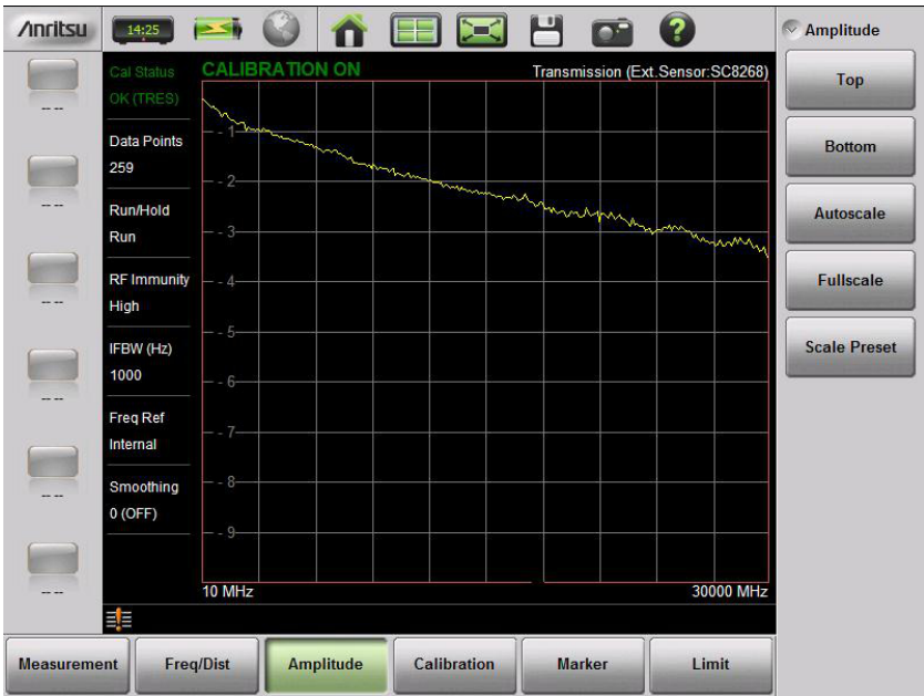
Figure 3-15. External Sensor Transmission Measurement Example
