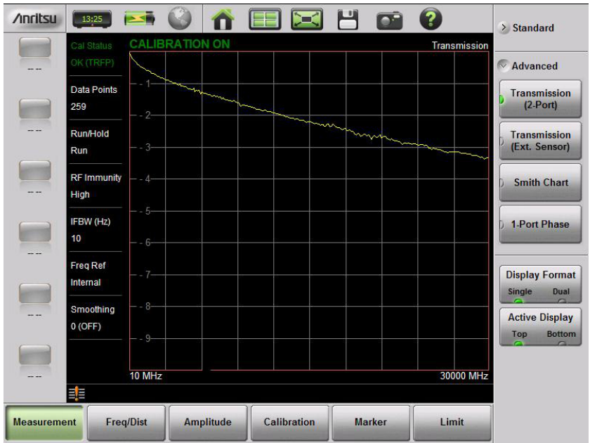
Figure 3-14. 2-Port Transmission Cable Loss Measurement Example
