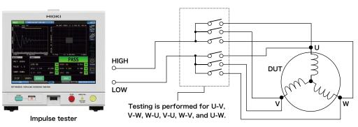
Fig. 2 Impulse testing of a 3-phase stator
