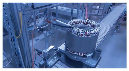
Fig. 1 Testing a stator
