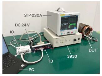
Fig. 3 Photograph of measurement and control equipment
