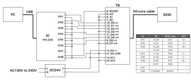
Fig. 6 Relay control wiring diagram
