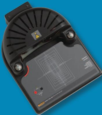
The **52120A/COIL3KA, COIL, 25 TURN, 3000 AMP** is a 12V-powered coil with a maximum compliance voltage rating of 4.5 volts RMS. With forced-convection cooling, it may run continuously at 120 amps, allowing it to calibrate clamp meters up to 3000 amps.
