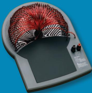
The **5500A/COIL 50-turn Current Coil** is a non-powered coil with a maximum compliance voltage rating of 3 volts RMS. At its rated current of 20 amps, it can calibrate clamp meters up to 1000 amps. It may run continuously to 11 amps, and must observe a 20% duty cycle from 11 amps to 20 amps.
