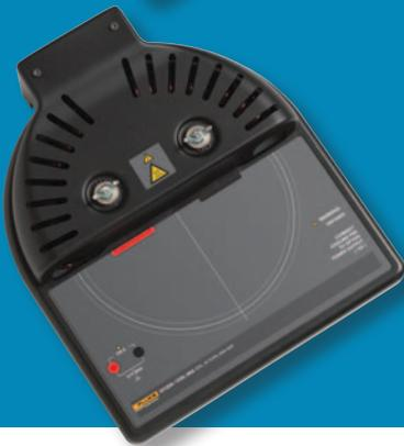
The **52120A/COIL6KA, COIL, 50 TURN, 6000 AMP** is a 12V-powered coil with a maximum compliance voltage rating of 4.5 volts RMS. Also convectively cooled, it may run continuously at 120 amps, allowing it to calibrate interruptible Rogowski coils, of lengths greater than 18 inches, at up to 6000 amps.
