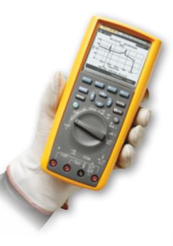
recommended mode when testing According to Mr. Zemánek, their for absence or presence of live power). Even more basic measurements include the range of accessories that can be attached. These can be valuable when working in the field - Mr. Zemánek often uses the magnet (Fluke TPAK) for attaching the multimeter to an electrical cabinet.
