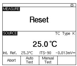
Figure 5. MEASURE/SOURCE split screen, contacts reset.
