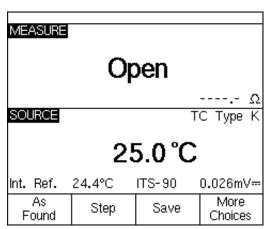
Figure 2. MEASURE/SOURCE split screen, contacts open.
