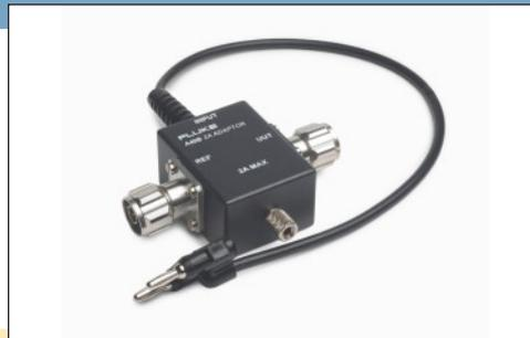
The low current adapter is used to calibrate shunts at currents levels of 2 A or less. It connects together the current source and two shunts for calibration measurements. This adapter mates with N-type connectors to the shunts and a dual banana connection to the source. In this configuration, a certified or reference shunt is connected in series with a shunt that is being calibrated, which in turn are in series with a current source.
