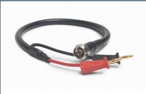
This lead permits connecting the A40B shunt's N-type connectors to instrumentation that uses dual banana plug connection terminals. Using two leads permits connecting the shunt's voltage output to a voltage measuring instrument and also connecting the shunt's current input to a UUT current source rated 20 A or less.
