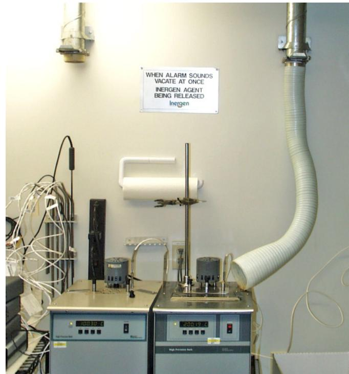
**Figure 1** Ventilation system for removing oil vapors.
